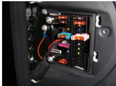
14. Snap fuse into any free slot
