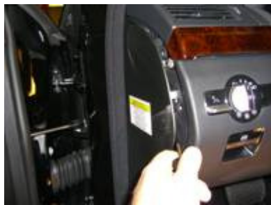
1. Pry left side fuse cover
