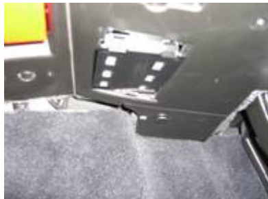
4. Locate CAN Distributor Panel
