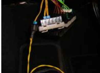
10. Connect Radio Plug to VIM221
