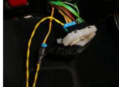
12. Completed CAN connections
