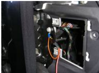
13. Connect ground lug to 10mm bolt
