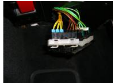
6. Unclip socket with yellow wires
