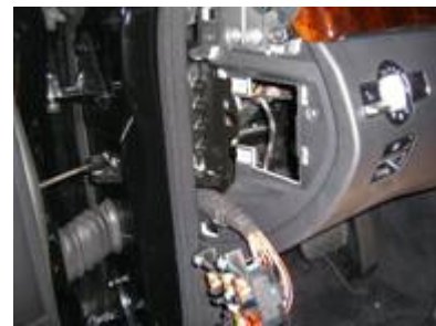
3. Remove Fuse Panel
